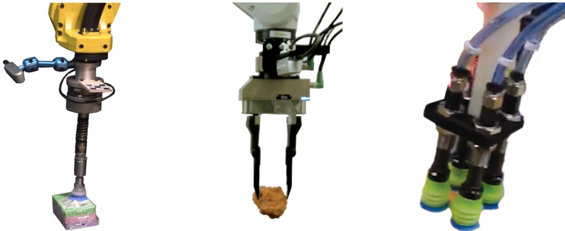
Exhibit 2b Example end effectors for gripping objects
